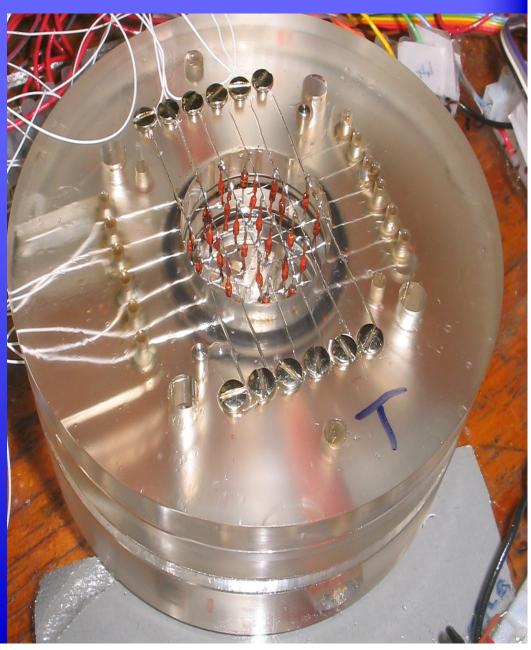
An array of diodes for the measurement of the mid-height temperature distribution
